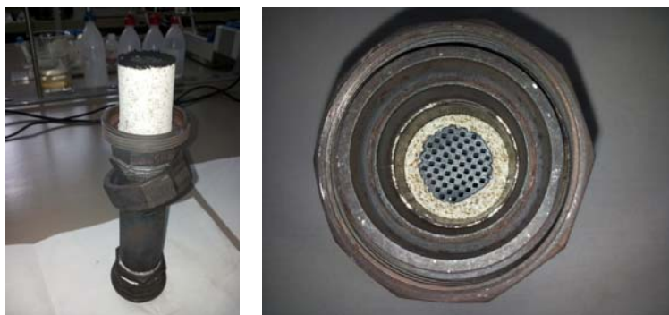
Figure 1: Filter housing and intumescent ceramic-mat wrapped around the filter.
