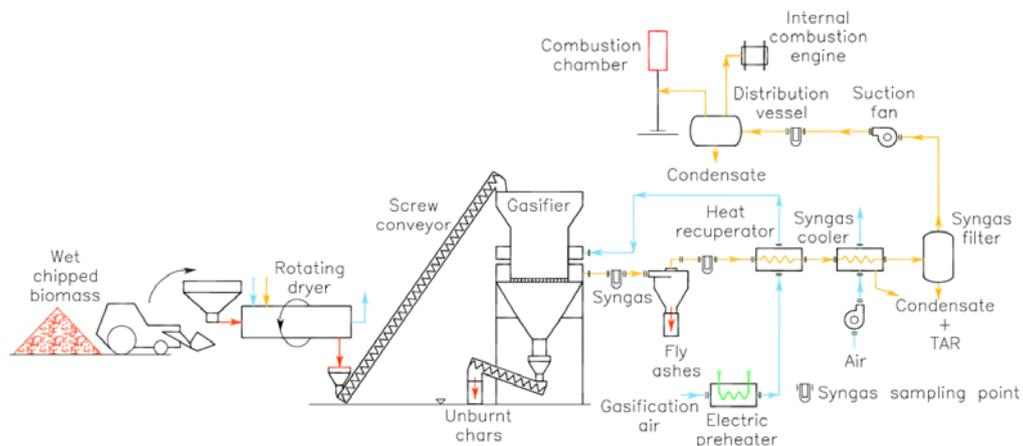
Figure 1: Schematic flowsheet of the full scale downdraft gasification plant
