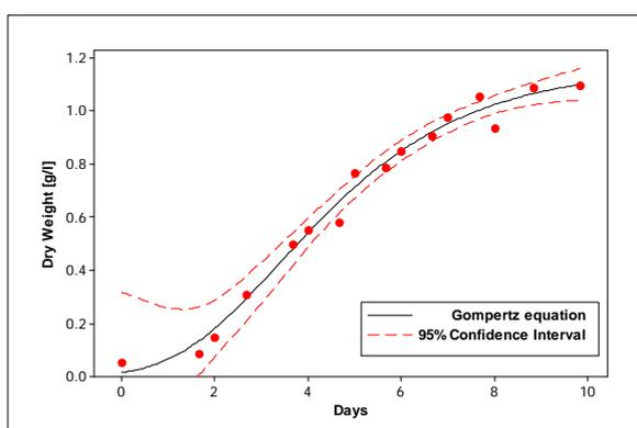
Figure 3: growth curve in terms of Dry Weight and fitted Gompertz equation
