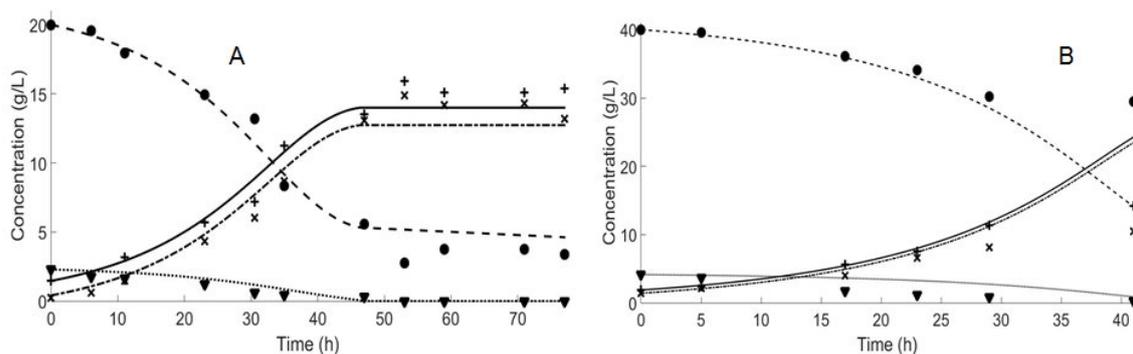
Figure 2. Results in batch bioreactor. A) 5 L fermentation with 20 g/L vegetal oil and B) 60 L with 40 g/L vegetal oil. Experimental data: ( $\nabla$ ) ammonium sulfate, ( $\bullet$ ) vegetal oil, ( $\times$ ) product PHA, (+) biomass and model prediction: (—) Biomass, (---) vegetal oil, (.....) ammonium sulfate, (-.-.) PHA.
