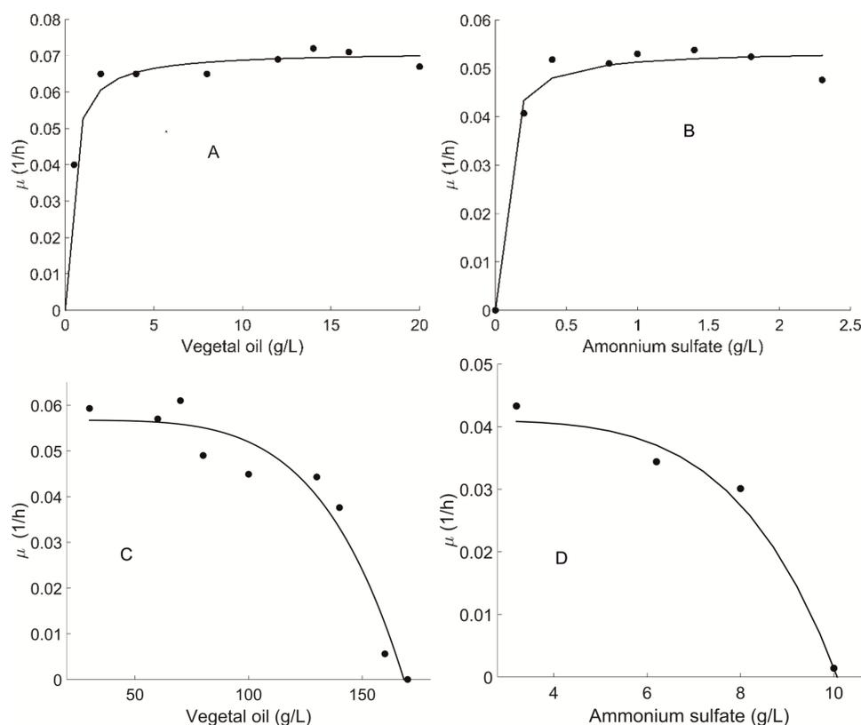
Figure 1. Behavior of specific growth rate ( $\mu$ ) as a function of concentration of limiting substrates. A) vegetal oil and B) nitrogen. And inhibiting substrates concentrations. C) vegetal oil and D) nitrogen. Smooth lines represent the fitted values (-), experimental data ( $\bullet$ ).
