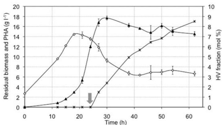
Figure 3: Evolution of the residual biomass (white rhombuses), PHA concentration (black triangle) and copolymer HV fraction (crosses) evolution during the fed-batch fermentation at bioreactor scale. Grey arrow indicates the feed switch from glucose to VFA mixture.
