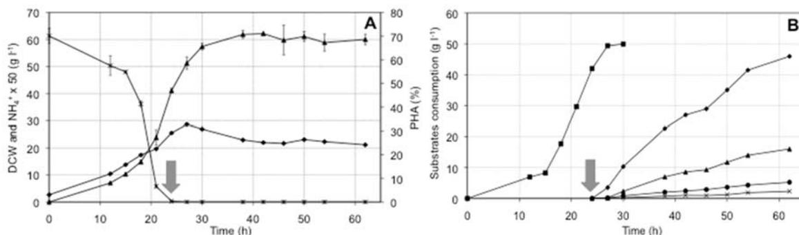
Figure 2: Time course of the PHA production at bioreactor scale. Figure A depicts the total dry cell weight production (rhombuses), PHA accumulation (triangles) and ammonia exhaustion (crosses). Figure B shows the consumption of carbon sources, glucose (squares), acetic (rhombuses), propionic (triangles), valeric (circles) and butyric (crosses) acid. Grey arrow indicates the feed switch from glucose to VFA mixture in both cases.
