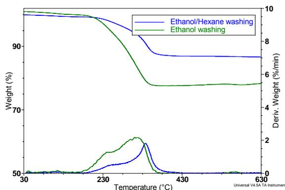
Figure 4: Thermogravimetric analysis of:  $\text{Fe}_3\text{O}_4$  nanoparticles washed with ethanol alone and  $\text{Fe}_3\text{O}_4$  nanoparticles washed with an equal volumetric ratio mixture of ethanol and hexane.
