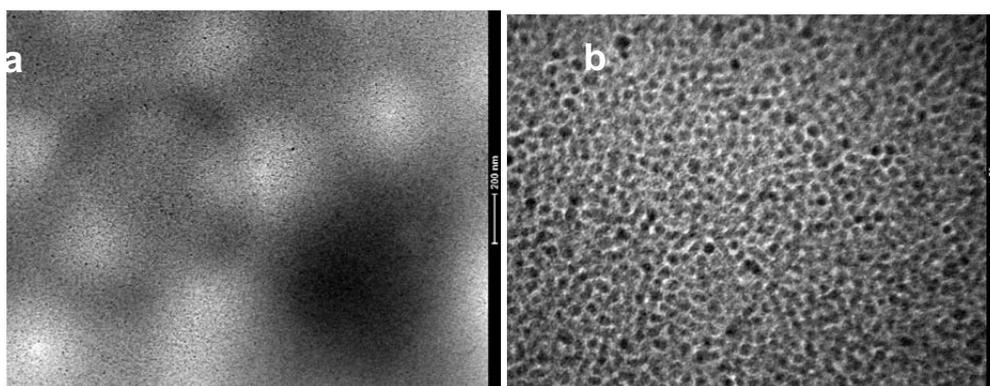
Figure 1: TEM images of  $\text{Fe}_3\text{O}_4$  nanoparticles at different magnification
