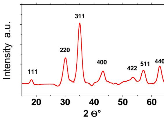
Figure 2: XRD pattern of synthesized  $\text{Fe}_3\text{O}_4$  nanoparticles
