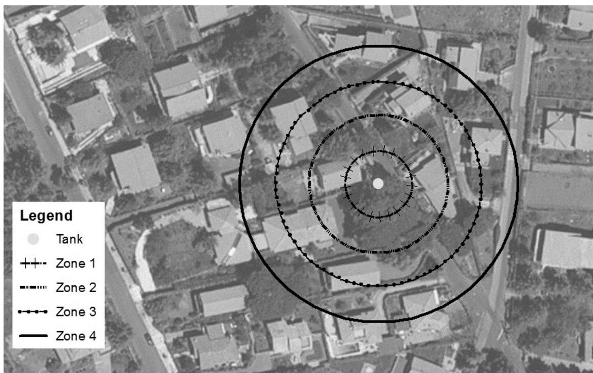
Figure 3. Damage zones for a water BLEVE.
