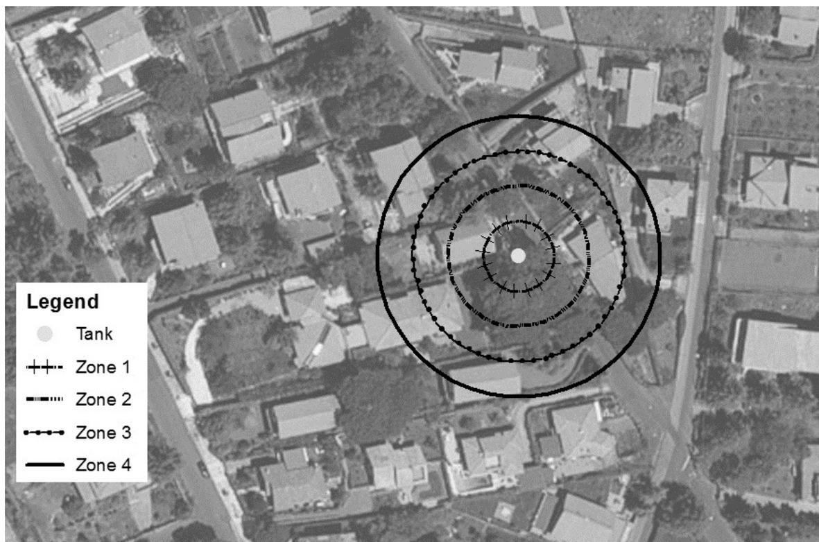
Figure 2. Damage zones for a LPG BLEVE.
