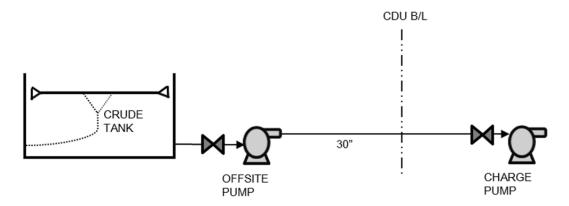
Figure 4: Pumps operating in series, with long suction header
