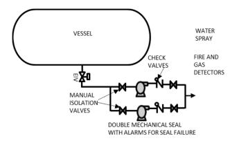
Figure 1: Typical depiction of an LPG Vessel and associated pump
