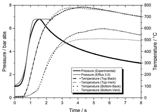
Figure 3: Measured pressure- and temperature-time profiles for a gas mixture consisting of 11 vol.% methane in air, centrally ignited in a closed  $5 \text{ m}^3$  vessel at an initial pressure of 1 bar abs and an ambient initial temperature, and a pressure-time profile as predicted by the Efflux method.
