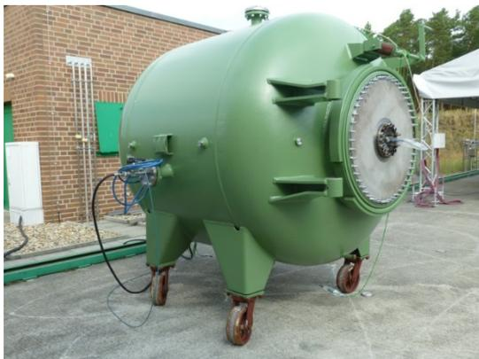
Figure 2: Test vessel with inner volume of 5 m<sup>3</sup> ( $L/D = 1.18$ ); official pressure rating of 30 bar abs at 20 °C.
