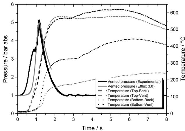
Figure 4: Pressure- and temperature-time profiles for a gas mixture consisting of 11 vol.% methane in air, centrally ignited in a  $5 \text{ m}^3$  vented vessel ( $F = 0.0113 \text{ m}^2$ ,  $p_{\text{stat}} = 1.9 \text{ bar abs}$ ) at an initial pressure of 1 bar abs and an ambient initial temperature, and a vented pressure-time profile as predicted by the Efflux method.
