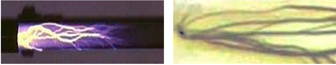
Figure 1: Propagating brush discharge and traces of propagating brush discharges in a transparent plastics pipe.
