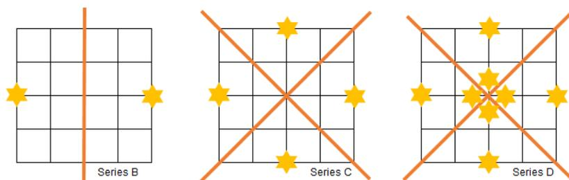
Figure 5: Sectioning of explosion cells for multi-ignition point experiments B, C and D
