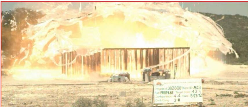
Figure 3 above shows a snapshot of the fully developed flame during single ignition point experiment A03, 340 msec after ignition at the left side.
