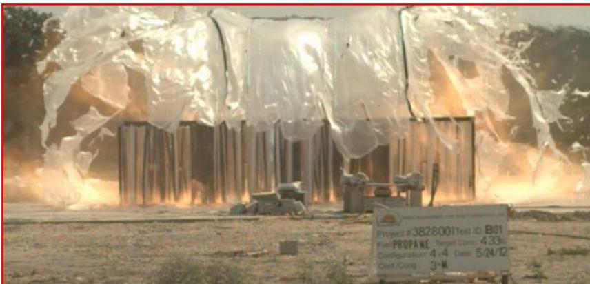
Figure 4 above shows the fully developed flame during 2-ignition point experiment B01 at 370 msec after simultaneous ignitions at the left and at the right sides
