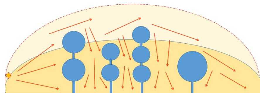
Figure 8: Flame propagation through an arrangement of exchangers with vertical barriers between the shells.
