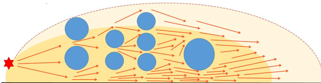
Figure 7: Flame propagation through an arrangement of heat exchangers
