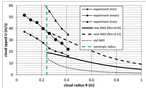
Figure 4: Cloud speed validation against Pettitt experiments (Freon 11, 100% fill, 4.10 barg, 1 litre)
