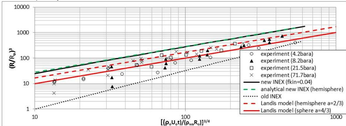
Figure 2: Validation of cloud volume versus time against Landis nitrogen experiments
