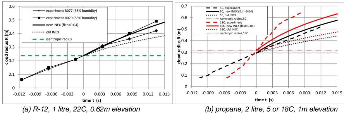
Figure 5: Cloud radius versus time for Schmidli experiments (100% fill)
