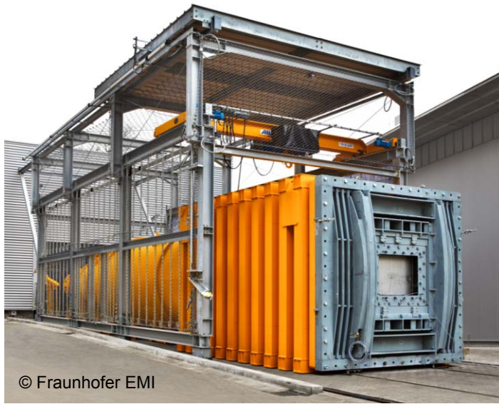
Figure 2: View on expansion chamber of the Blast-STAR facility with the end-section wall (grey) for the integration of test samples.
