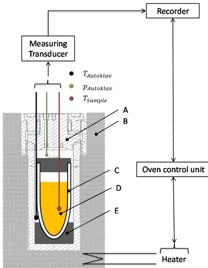
Figure 1: Schematic drawing of the test set-up, with A) autoclave, B) block furnace, C) Dewar vessel, D) test item, E) insulation material
