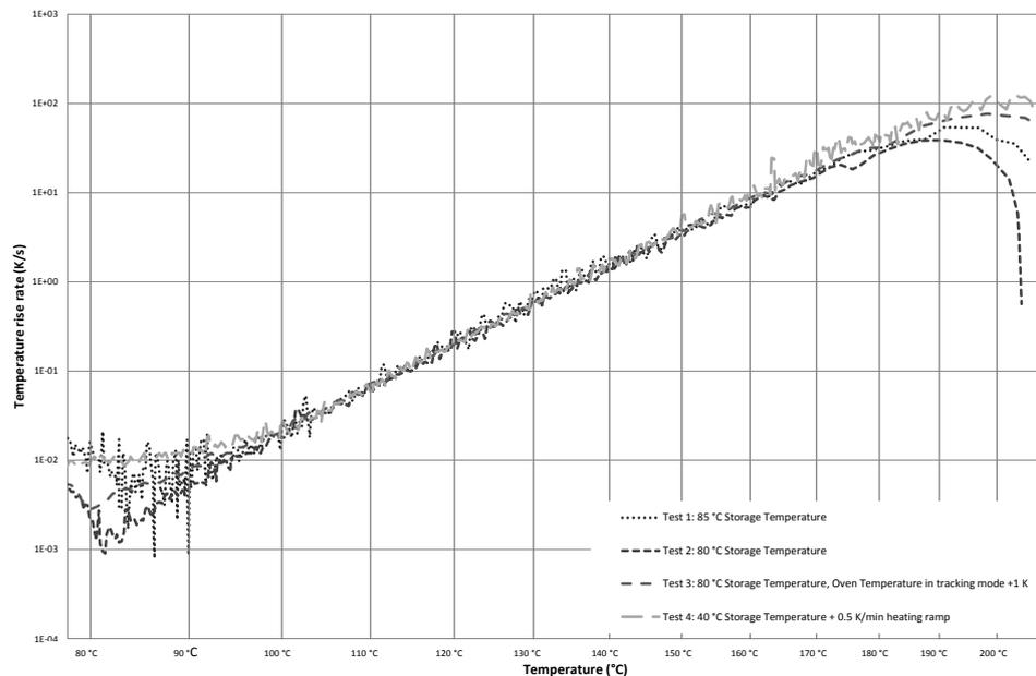
Figure 3: Temperature rise rate as a function of the reciprocal, absolute temperature for all four experiments. For the graphical representation the reciprocal, absolute temperature values of the x-axis are replaced by the corresponding temperatures in degrees Celsius.
