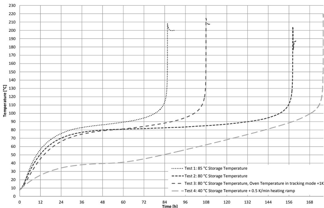
Figure 2: Courses of the temperature dependent on the measuring time for all four experiments.
