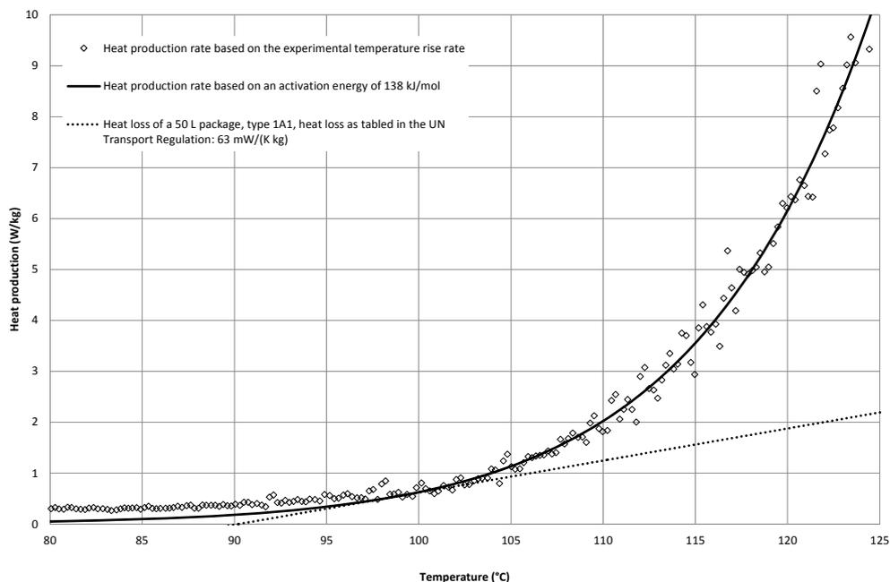
Figure 4: Exemplary determination of the SADT in the Semenov plot. The heat production rate is calculated by using a heat capacity of the reaction system of 1900 J/(kg•K).
