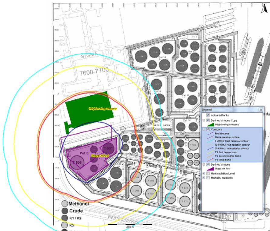
Figure4: Heat load calculations of pool fire within a tank pit
