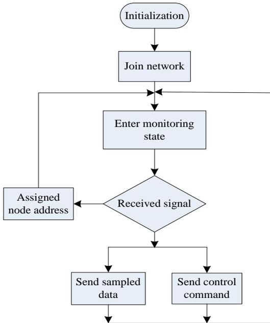
Figure 5: The flow chart of router node
