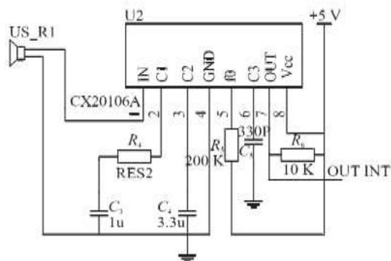
Figure 3: The ultrasonic receiving circuit
