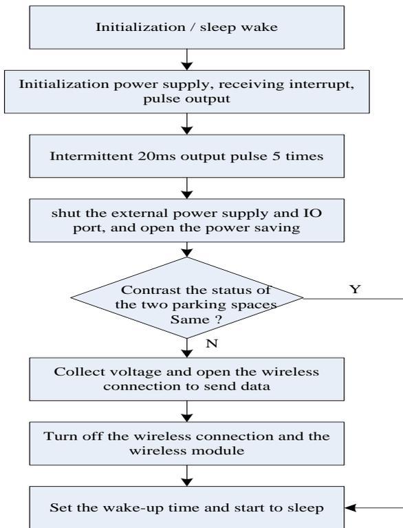
Figure 7: Parking detection flow chart
