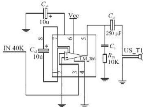
Figure 4: The ultrasonic transmitting circuit
