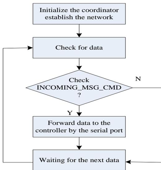
Figure 6: The flow chart of the coordinator
