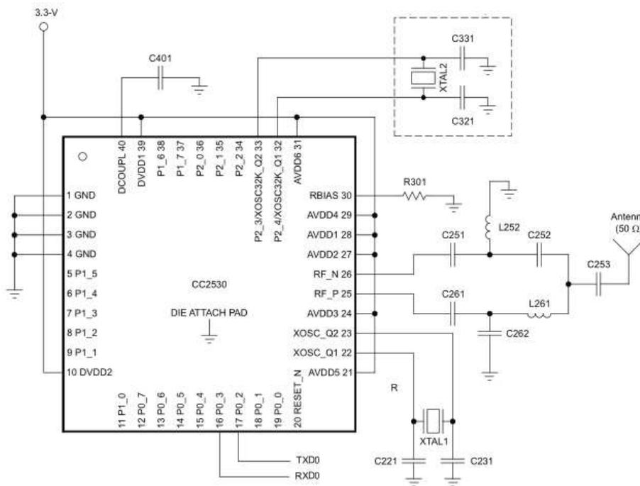
Figure 2: Design of the Zigbee circuit
