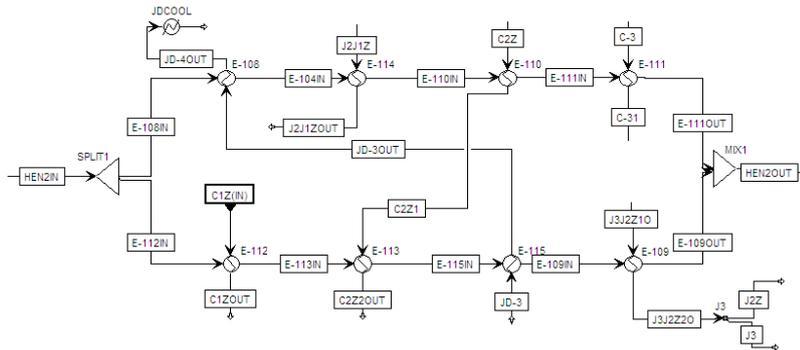
Figure 2: The heat exchanger network between the desalination and the flash column (HEN2). JD-3, JD-4 -The residue of the VDU; J2J1Z, J3J2Z - the first and the second pumparound of the VDU; C1Z, C2Z, C3 - The first, second and the third pumparound of the ADU
