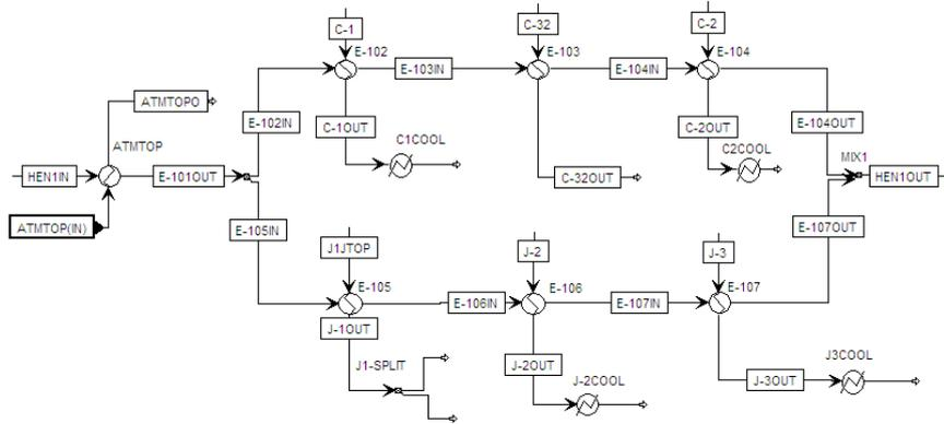
Figure 1: The HEN before desalination (HEN1). CRUDE - Crude Oil, C1, C2, C32 - the first, second and the third side draw of the ADU; J1JTOP, J2, J3 - the first, second and the third side draw of the VDU
