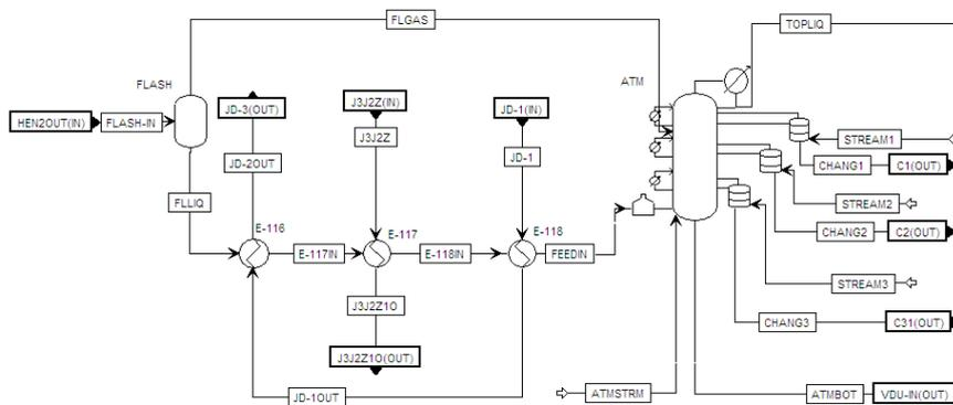
Figure 3: The HEN between the flash and the ADU column (HEN3) and the ADU. JD-1, JD-2 - The residue of the VDU; J3J2Z - The second pumparound of the VDU
