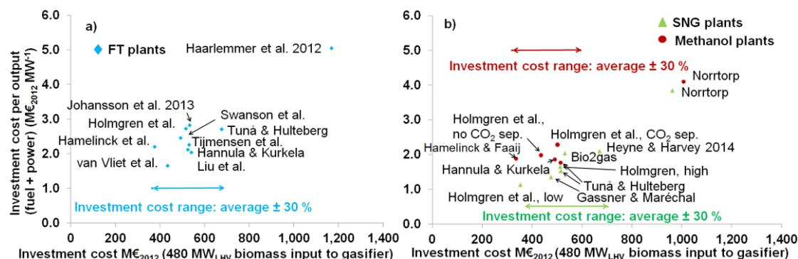
Figure 1: Comparison of total plant investment cost estimates for FT systems (a) and SNG and methanol systems (b).
