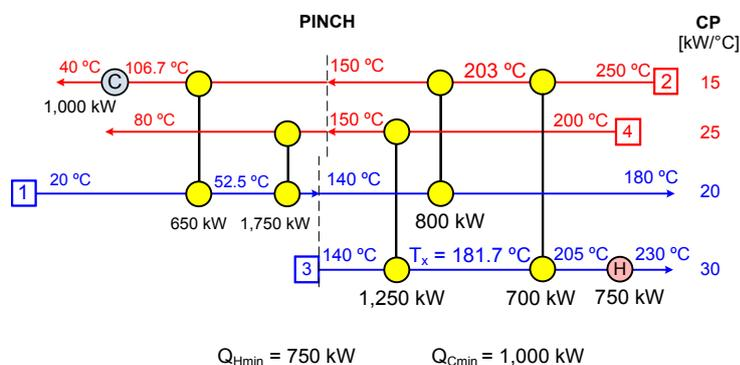
Figure 1: Grid Diagram for the a HEN (adopted from Klemeš et al., 2014)
