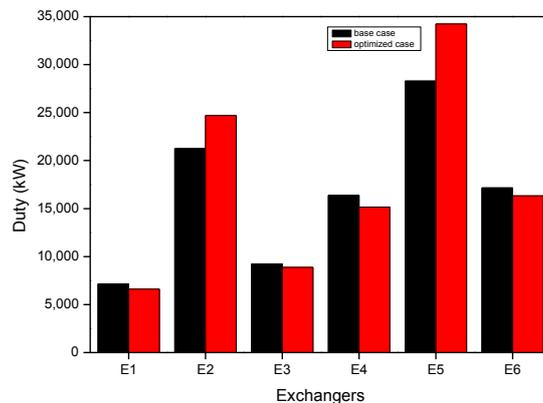
Figure 3: Comparison of duty in base and optimized cases
