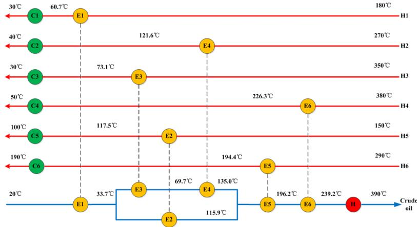
Figure 1: Heat exchanger network configuration in crude oil preheat train
