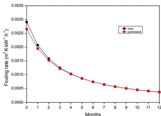
Figure 4: Fouling rates of E6 in base and optimized cases
