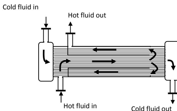
Figure 1: 2-1 Pass helical baffle heat exchanger.
