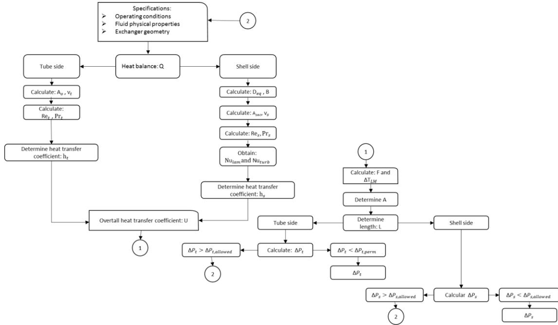
Figure 3: Flow diagram of the design approach.
