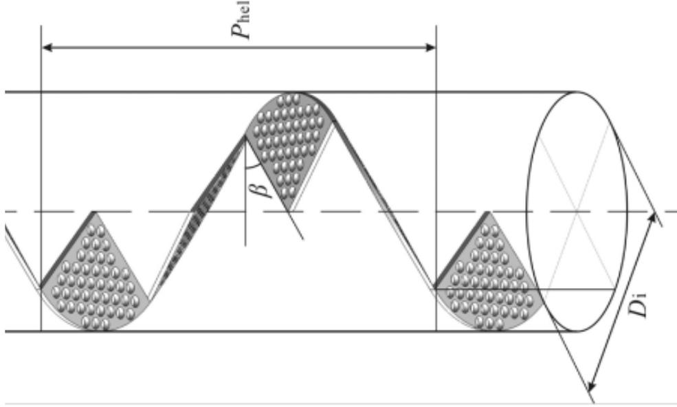
Figure 2: Main geometrical features of a helical baffle exchanger.
