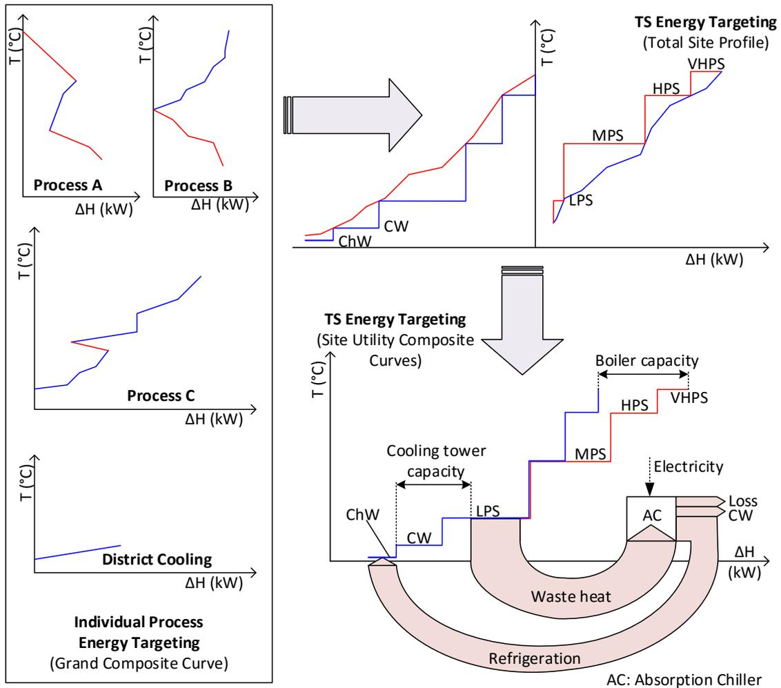
Figure 2: TS energy targeting with absorption chiller
