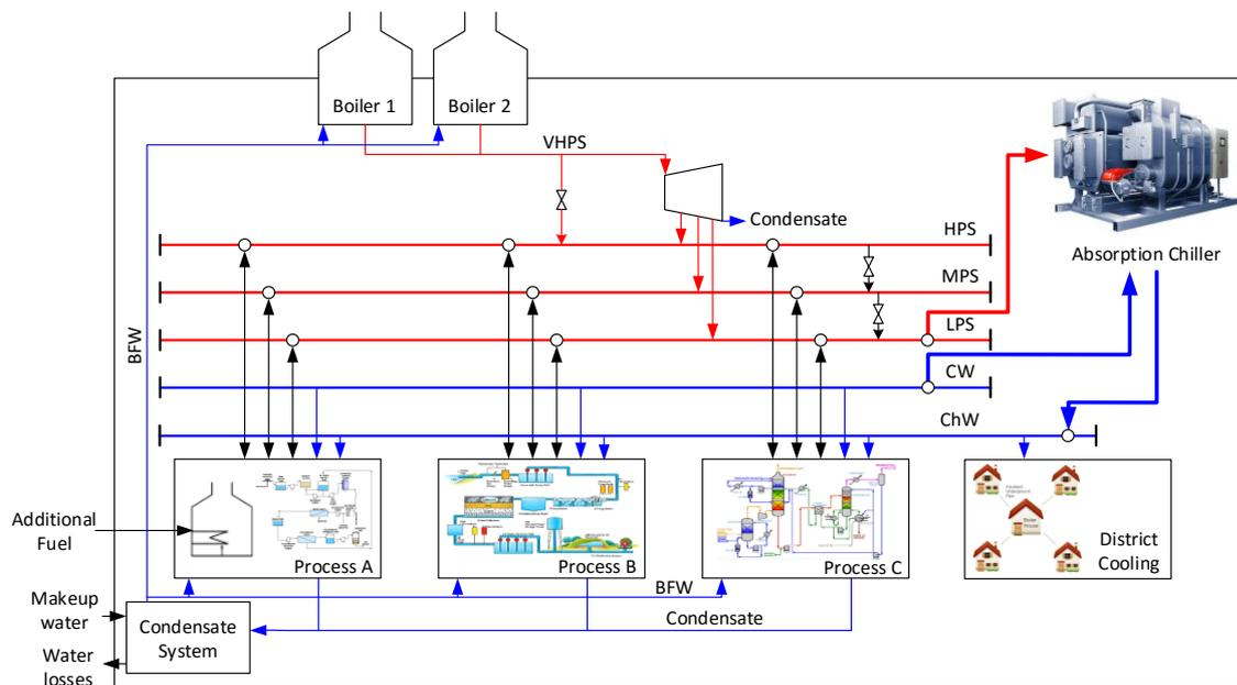
Figure 1: A Total Site with an integrated centralised cooling system
