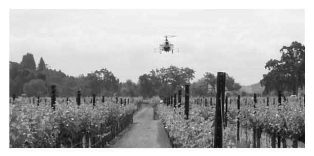
Figure 2. Unmanned aerial vehicle (UAV) spray pass over vineyard as viewed by aircraft operator
