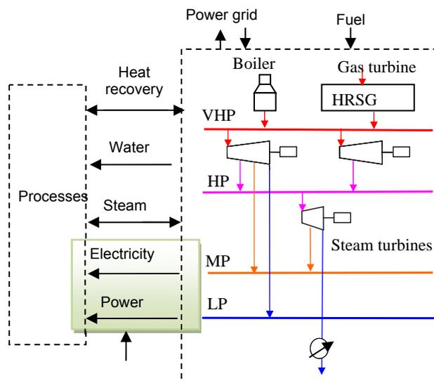
Figure 1: Utility system superstructure
