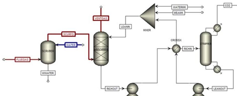
Figure 1: Simplified process flow diagram of MEA-based scrubbing system (Aspen plus).
