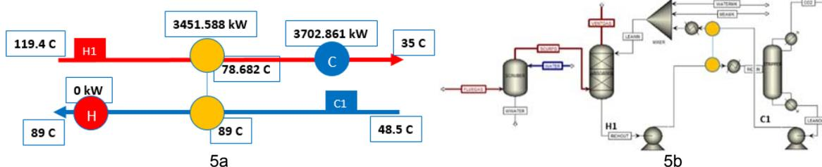
Figure 5a and 5b: Conceptual process integration from GAMS and validated process flow diagram of improved MEA-based scrubbing system (Aspen plus) with process heat integration.
