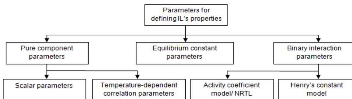
Figure 2: Flowchart of defining ionic liquid into Aspen Plus (Khonkaen, et al., 2014).
