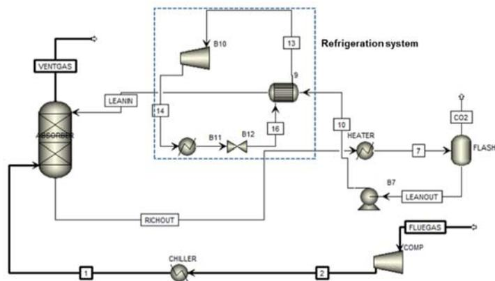
Figure 3: Simplified process flow diagram of IL-based scrubbing system (Aspen plus).
