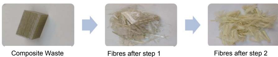
Figure 2: UP composite from experiment 3. Appearance after step 1 and appearance after step 2
