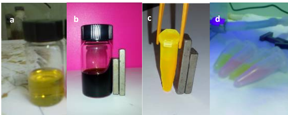
Figure 6: Photograph showing the high stability in water of \text{Fe}_3\text{O}_4(\text{FITC})@\text{SiO}_2\text{-NH}_2 (a). Magnetism of \text{Fe}_3\text{O}_4 nanoparticles (b) and of \text{Fe}_3\text{O}_4(\text{FITC})@\text{SiO}_2\text{-NH}_2 (c) in response to a Gd magnet. Fluorescence photographs of \text{Fe}_3\text{O}_4(\text{FITC})@\text{SiO}_2\text{-NH}_2 in water under a UV lamp ( \lambda=365 \text{ nm} ) (c). *(the Eppendorf in pink contains a water solution of \text{Fe}_3\text{O}_4(\text{RBITC})@\text{SiO}_2\text{-NH}_2 , the fluorescent molecules are rhodamine-B-Isothiocyanate, RBITC)
