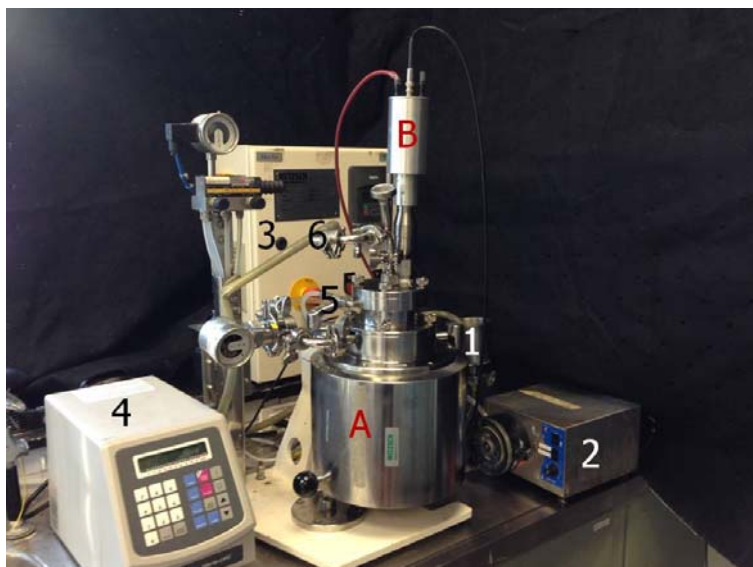
Figure 1: Mini-fer ball mill with an ultrasonic probe
