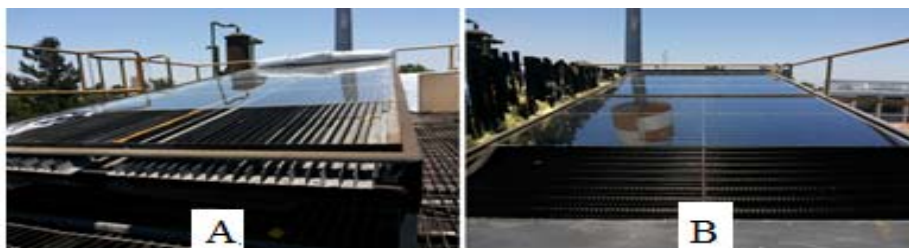
Figure 1: Hybrid solar dryer. A: Solar panel, B: Solar energy accumulator
