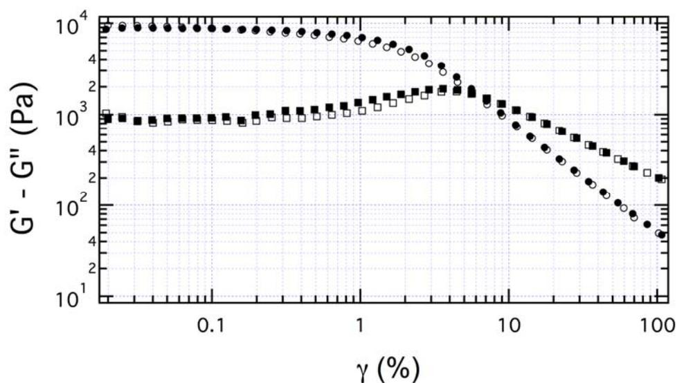
Figure 1: Strain dependence of the storage modulus ( $G'$ , circles) and loss modulus ( $G''$ , squares) of water dispersion of cell wall materials at 4.7% weight concentration. The test shows the existence of reversible stress softening (filled symbol and empty simple are the first and the second part of the test)
