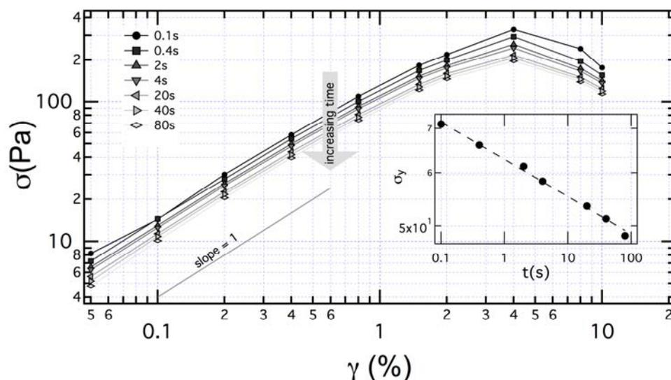
Figure 3: Double logarithmic representation of the shear stress-shear strain of the 4.7% cell wall particles dispersion extracted from stress relaxation data. Continuous line depicts slope 1 regime. Inset: yield stress values corresponding to each time
