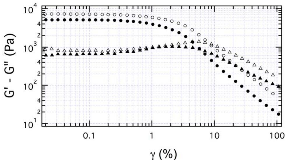
Figure 5: Strain dependence of the storage modulus ( $G'$ , circles) and loss modulus ( $G''$ , triangles) of water dispersion of crude apple tissue obtained from fresh (filled symbols) and ripe apple fruit (empty symbols)
