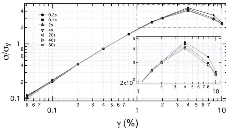
Figure 4: (main body) Normalization of shear stress data by yield stress ( $\sigma_y$ ). (inset) Magnification of the  $1\% < \gamma < 10\%$  region, showing the non superposition of the stress-strain data
