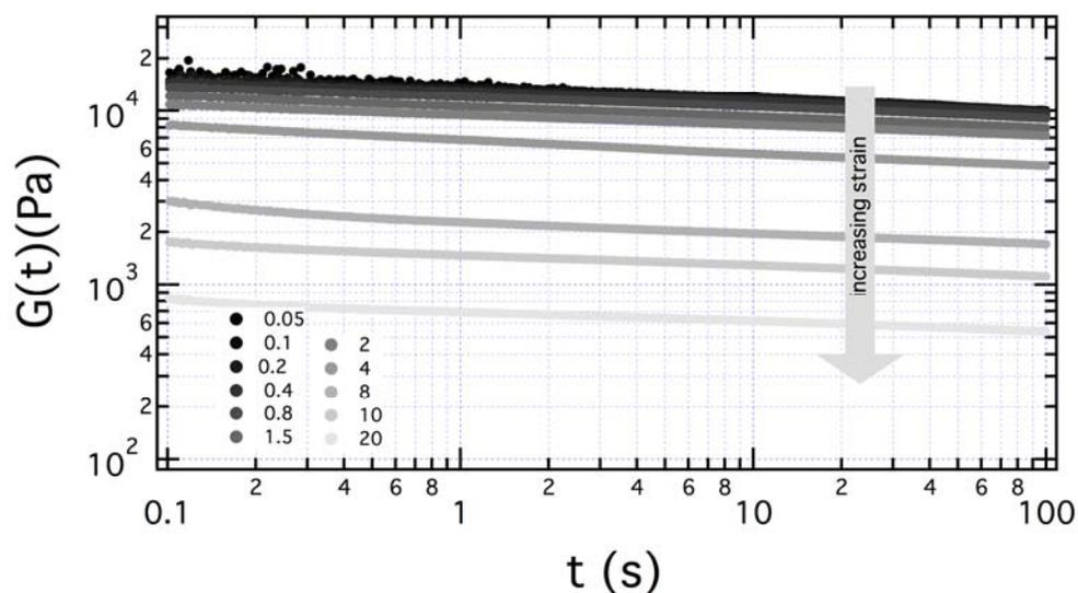
Figure 2: single step stress relaxation data for the 4.7% w/w cell wall particle dispersion in water. Different curves were obtained at different strains, as indicated in the legend
