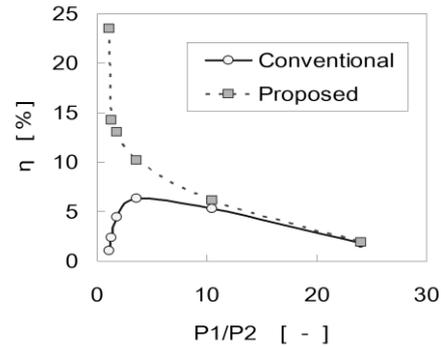
Figure 7: Comparison of the efficiency of power generation at different flash rates ( $P1/P2$ ) of the flash evaporator (working fluid: toluene, temperature in evaporator: 150 °C, temperature in condenser: 40 °C)
