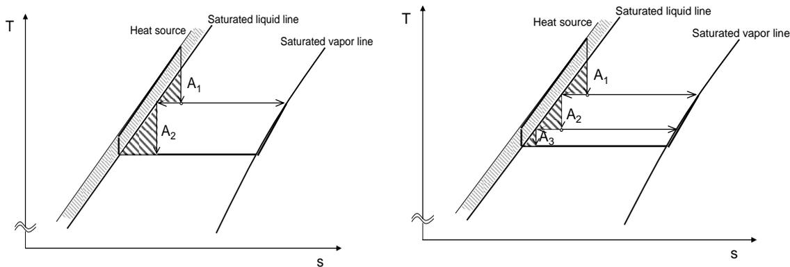
Figure 10:  $T$ - $s$  diagrams for the OFC system (left: single flash, right: double flash)
