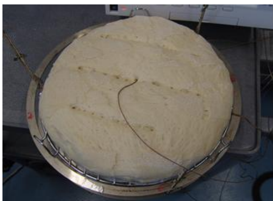
Figure 1: experimental configuration: bread and thermocouples in the centre
