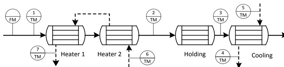
Figure 1: Layout of the pilot scale plant simulated. FM=flow measure, TM=temperature measure
