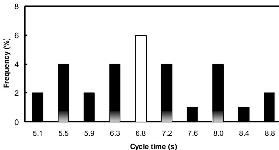
Figure 2: Cycle time distribution for a given system. Experimental conditions:  $\gamma$ ,  $28^\circ$ ;  $L_H$ , 0.15 m;  $D_T$ , 0.05 m;  $D_0$ , 0.04 m;  $H_0$ , 0.27 m;  $d_p$ , 0.006 m; material, glass beads.
