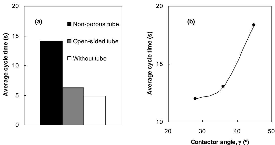
Figure 4: a) Overall average cycle times for the three systems studied, b) Influence of contactor angle of non-porous tubes on the average cycle time. Experimental conditions:  $L_H$ , 0.07 m;  $D_T$ , 0.05 m;  $D_O$ , 0.05 m;  $H_0$ , 0.27 m;  $d_p$ , 0.006 m; material, glass beads
