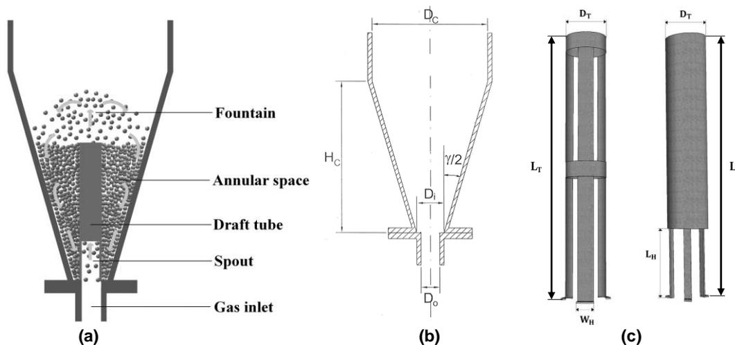
Figure 1: a) Zones in the conical spouted bed with conventional non-porous draft tube, b) geometric factors of conical spouted bed contactors and c) open-sided draft tube configuration and non-porous draft tube configuration.
