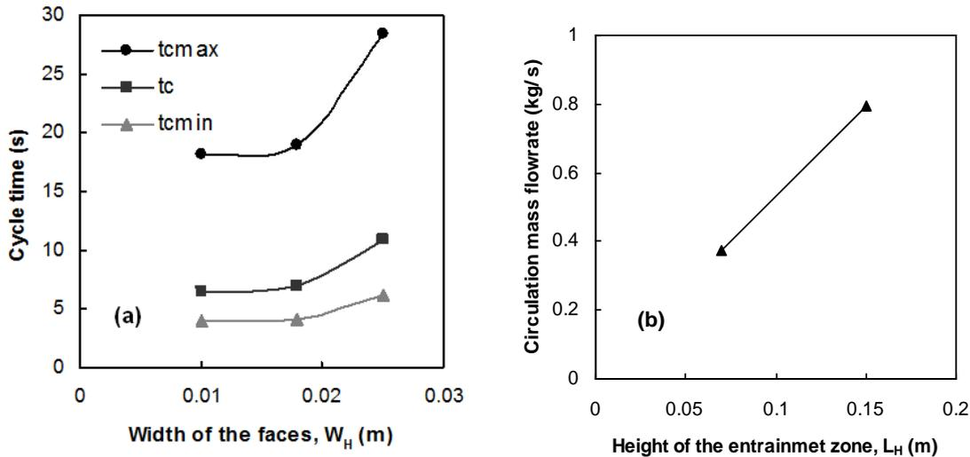
Figure 3: a) Influence of the width of the faces of open-sided tubes on the average, maximum, and minimum cycle times. Experimental conditions:  $\gamma$ , 36°;  $D_T$ , 0.04 m;  $D_o$ , 0.05 m;  $H_o$ , 0.27 m;  $d_p$ , 0.006 m; material, glass beads, b) Influence of the height of the entrainment zone of non-porous tubes on the solid circulation mass flowrate. Experimental conditions:  $\gamma$ , 28°;  $D_T$ , 0.04 m;  $D_o$ , 0.04 m;  $H_o$ , 0.17 m;  $d_p$ , 0.004 m; material, glass beads.
