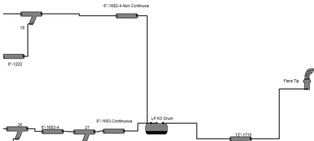
Figure 3: Part of LP flare network simulation area in FLARENET software
