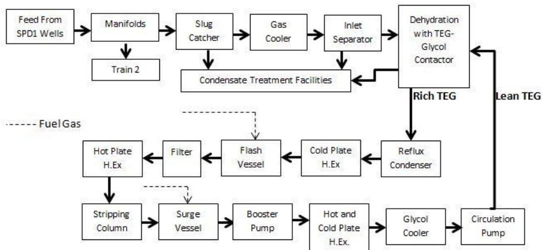
Figure 1: Process Block Diagram of main process facilities and GRU of phase 1 platform
