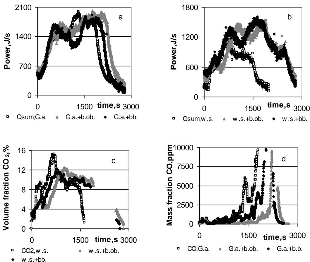
Figure 2: The effect of birch bark and birch outer bark addition to biomass on the time-dependent variation of heat power and composition of the products for wheat
