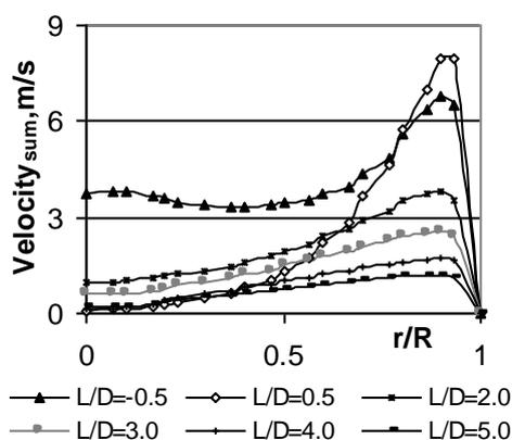
Figure 1: The formation of the swirling flow velocity profiles downstream the combustor
