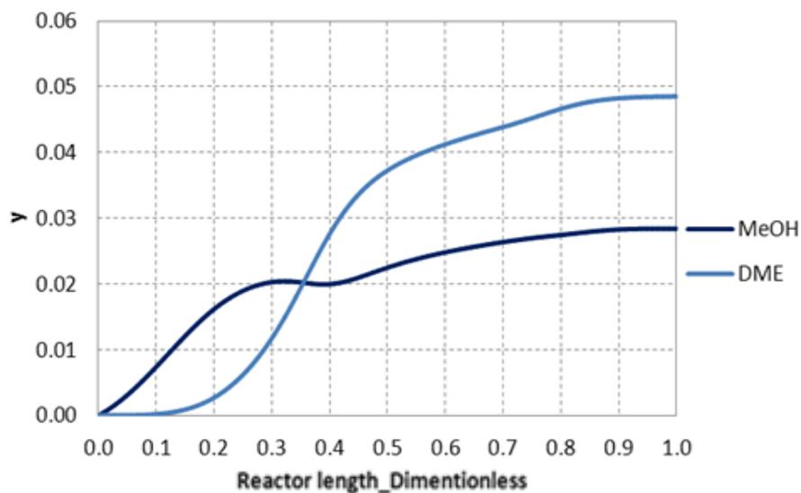
Figure 5: Methanol/DME production from the designated and proposed plant
