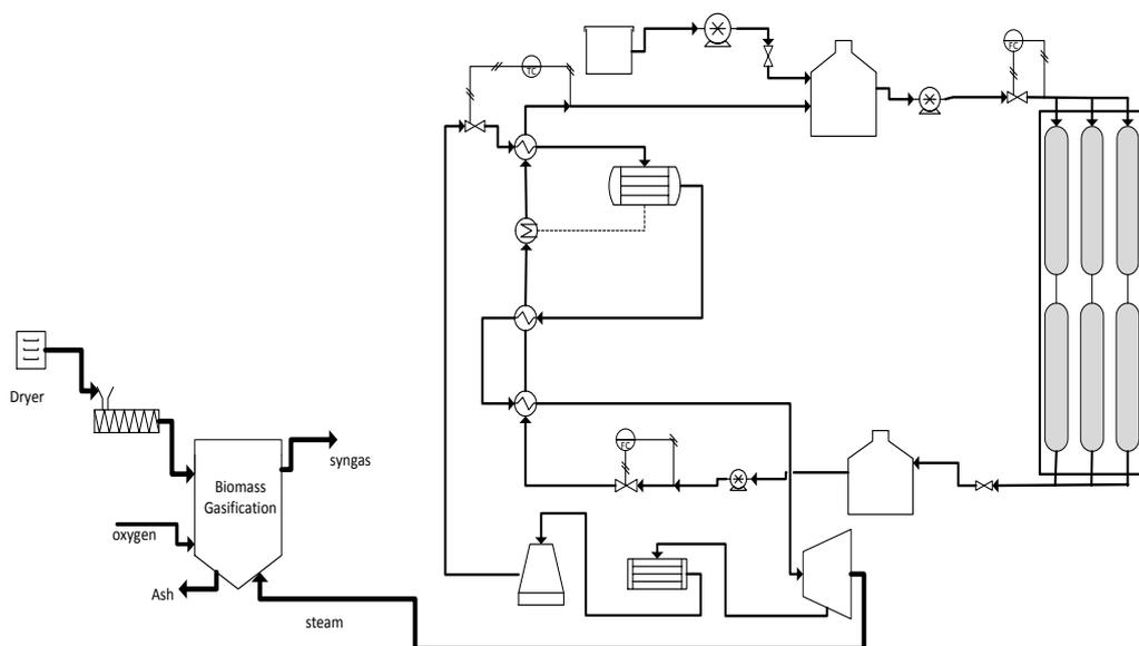
Figure 3: Flowsheet of the integrated biomass gasification with a concentrated solar power (CSP) plant
