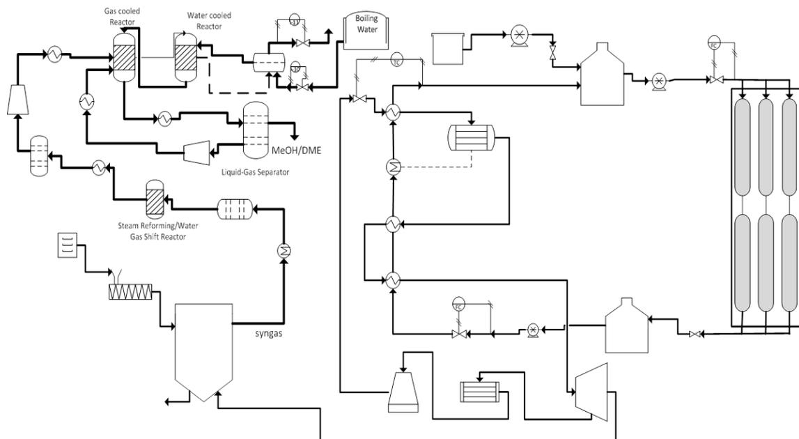
Figure 4: Flowsheet of biomass-to-methanol/DME process (the renewable pathway)
