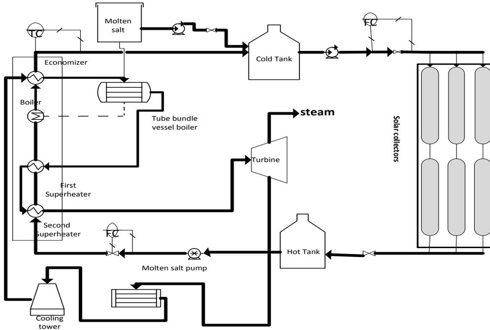
Figure 1: Flowsheet of the concentrated solar power (CSP) plant for power generation
