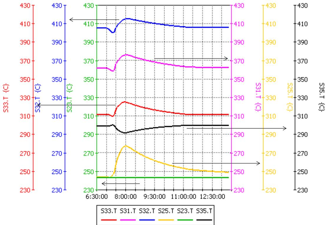
Figure 2: Temperature profile of: (S23.T) fresh water supplied to the heat exchange network; (S35.T) water outflowing the economizer; (S33.T) steam outflowing the boiler; (S31.T) steam outflowing the first superheater; (S32.T) steam outflowing the second superheater; and (S25.T) expanded steam leaving the turbine and sent back to the economizer
