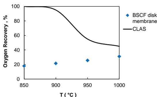
Figure 3: Comparison between the calculated oxygen recovery of the BSCF disk membrane and the CLAS process
