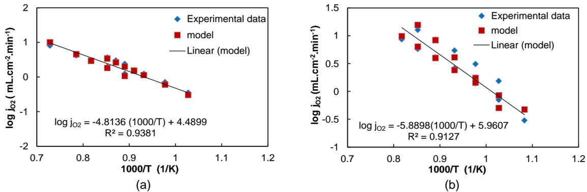
Figure 2: Logarithmic function of oxygen permeation flux across BSCF disk membrane for (a)  $L=1.5$  mm and (b)  $L=1$  mm
