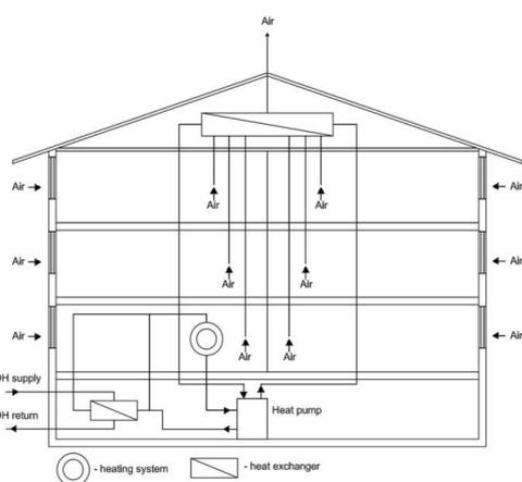
Figure 4: Basic schema of alternative 1
