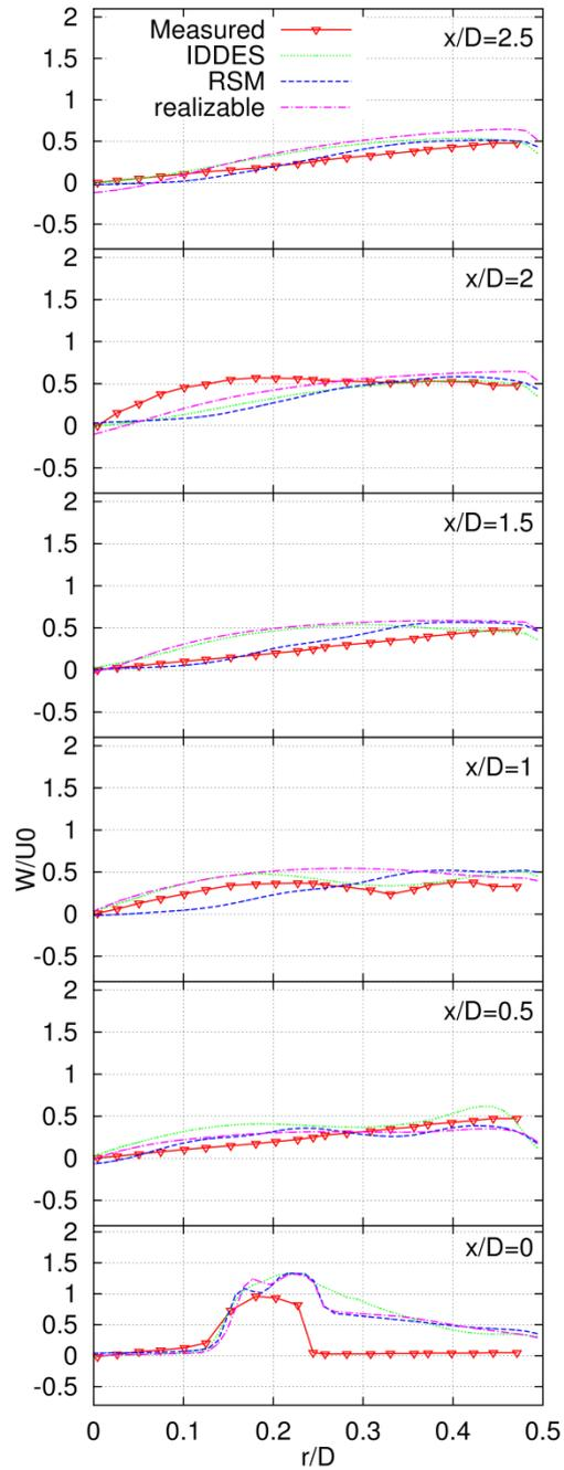
Figure 5: Tangential velocity profiles predicted by the three turbulence models validated with the measured data
