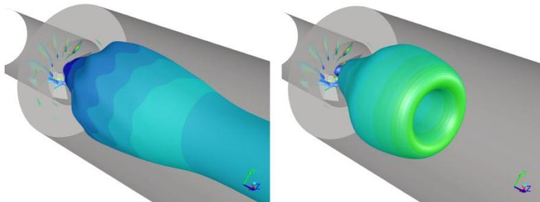
Figure 3: Internal recirculation zone of a) fully open outlet; b) partially blocked outlet
