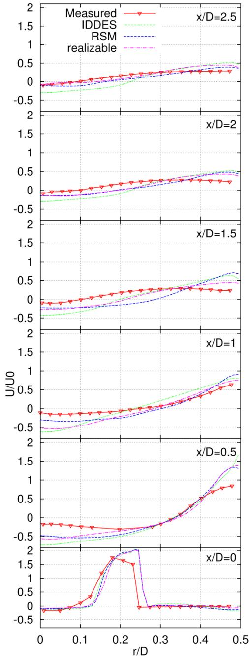
Figure 4: Axial velocity profiles of the three turbulence models validated with the measured data
