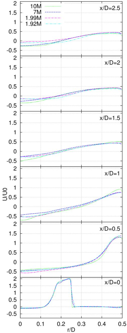
Figure 1: Velocity profiles of the grid independence study
