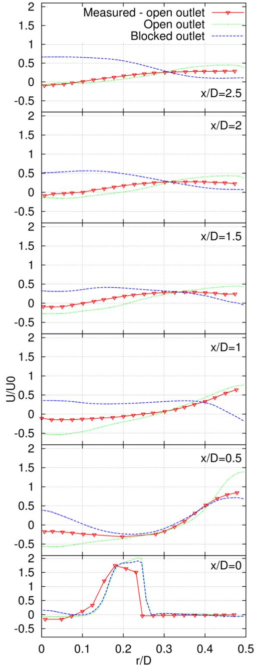
Figure 2: Influence of the outlet shape on the velocity profiles inside the chamber
