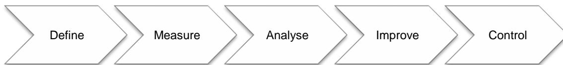
Figure 1: Systematic approach to optimise ovens for energy saving
