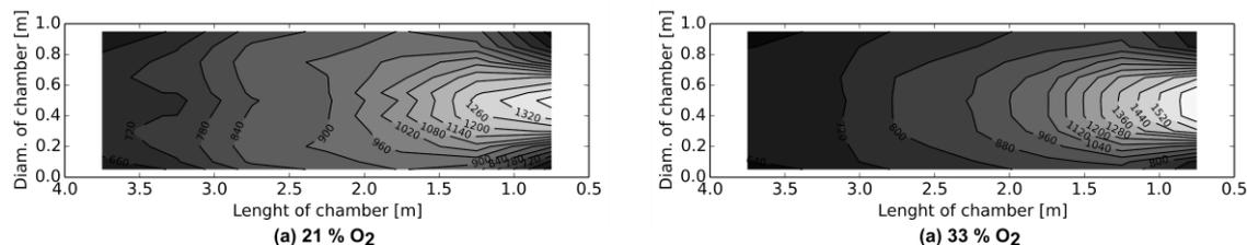
Figure 4: Temperature distribution for the PE one-staged combustion regime
