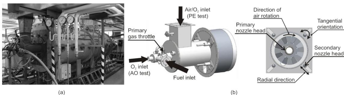
Figure 1: (a) The testing facility, and (b) the 3D model of experimental two-gas-staged burner
