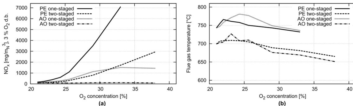
Figure 2: Effects of oxygen concentration on (a) NO<sub>x</sub> emissions and (b) flue gas temperature
