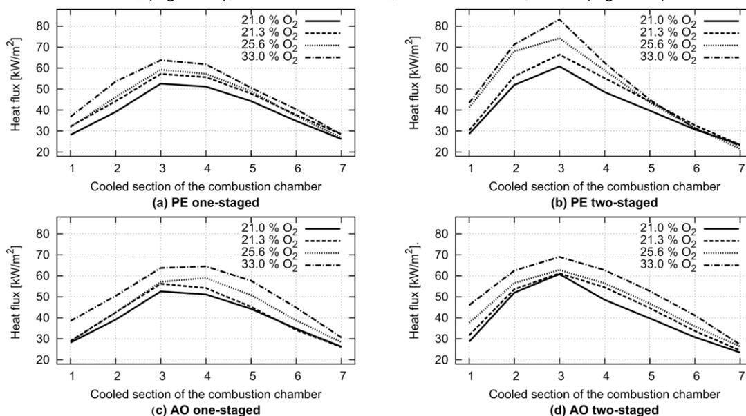
Figure 3: Heat flux profiles lengthwise the chamber at different oxygen concentrations
