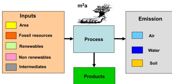
Figure 4: SPI calculation, material and energy flows of a process (SPIONWeb, 2014)
