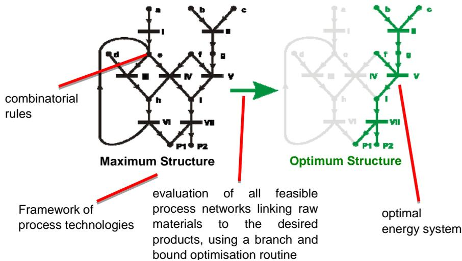
Figure 3: Maximum structure and Optimum structure of a technology network (Friedler et al., 1995, adapted)
