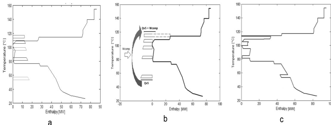
Figure 4: a) Preliminary GCC and evaporation system, b) Preliminary GCC and evaporation system with vapour bleeding at 1<sup>st</sup> effect and with vapour recompression of 5<sup>th</sup> effect, c) Final GCC
