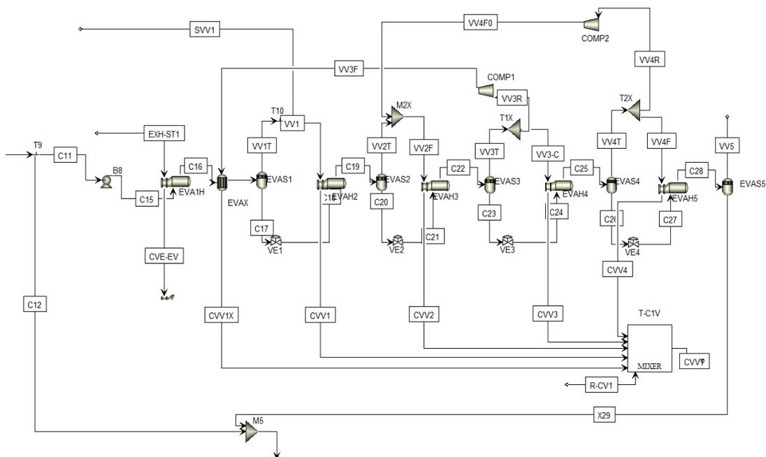
Figure 3: Flow sheet of the vapour recompression integrated to the evaporation system in Aspen® - Recompression of 3<sup>rd</sup> to 1<sup>st</sup> effect and 4<sup>th</sup> to 3<sup>rd</sup>
