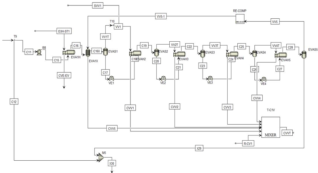
Figure 2: Flow sheet of the vapour recompression integrated to the evaporation system in Aspen Plus® - Recompression of 5<sup>th</sup> effect to 1<sup>st</sup> effect
