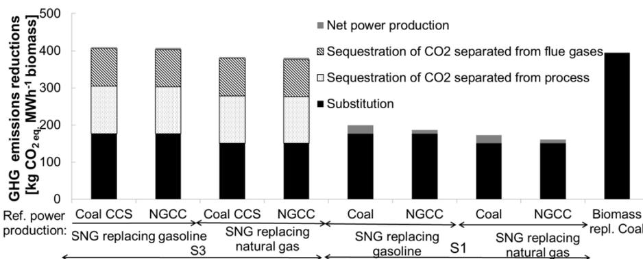
Figure 4: The GHG emission reductions with and without storage of separated CO<sub>2</sub> and for different reference power production technologies and fuels substituted by the SNG. The rightmost staple displays the reduction potential for using the biomass to replace coal in a condensing power plant
