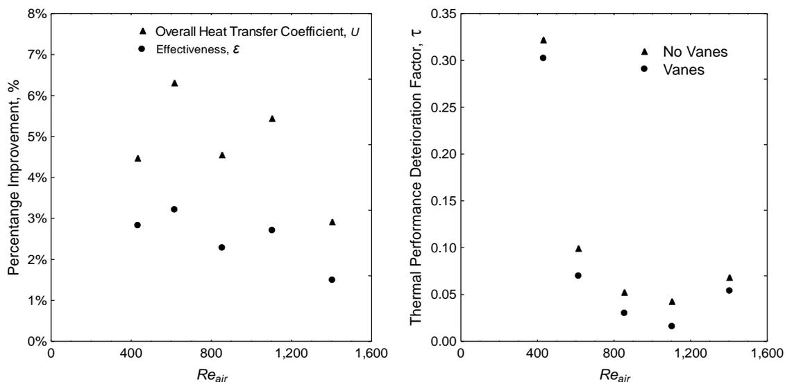
Figure 4: The percentage improvement in overall heat transfer coefficient and effectiveness by the addition of vanes (left) and the thermal performance deterioration factor with and without vanes (right) for a range of air-side Reynolds numbers
