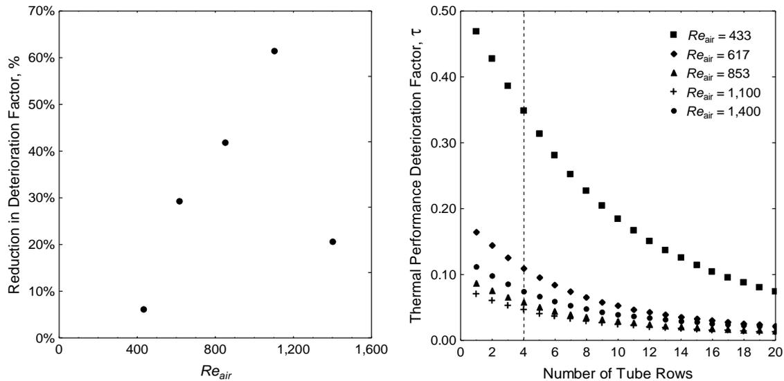
Figure 5: Percentage reduction in the thermal performance deterioration factor with the addition of vanes for a range of air-side Reynolds numbers (left) and the predicted effect of the number of tube rows on the thermal performance deterioration factor for each air-side Reynolds number tested (right)
