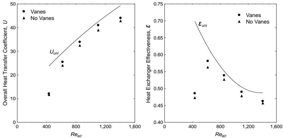
Figure 3: The overall heat transfer coefficient (left) and the heat exchanger effectiveness (right) for a range of air-side Reynolds numbers with vanes, without vanes, and the theoretical uniform case (solid line)
