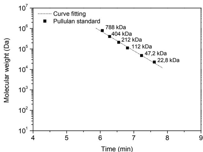
Figure 1: Molecular weight distribution of standard pullulan solutions (injection of 10  $\mu\text{L}$  at a concentration of 0.1 % w/V of each analytical standard in Ultrahydrogel Linear (300 mm x 7.8 mm column id) Waters brand with ultrapure water as mobile phase at a flow rate of 1.00 mL/min and conditioned at 80  $^{\circ}\text{C}$ ).
