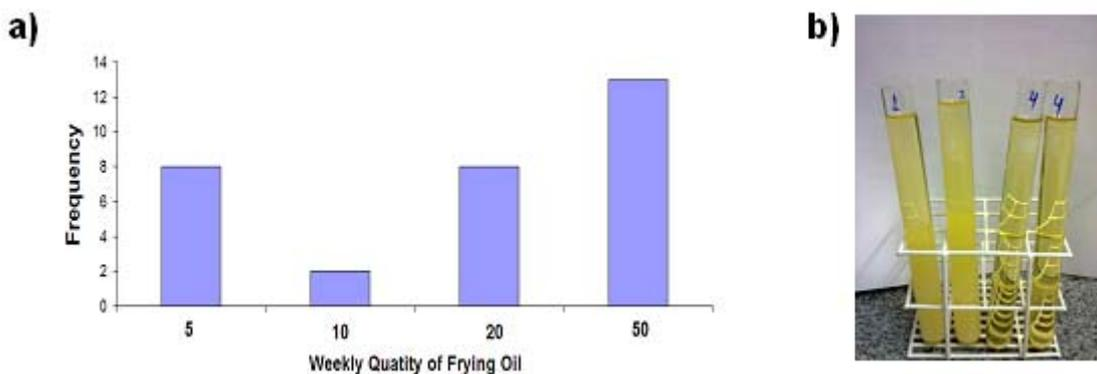
Figure 4: a) Responses of restaurant managers for weekly quantity of frying oil used, b) Photo of biodiesel from restaurant frying oils before and after filtration
