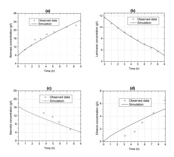
Figure 1: Observed data and simulation profiles for biomass (a), laminaran (b), mannitol (c) and ethanol (d) concentrations
