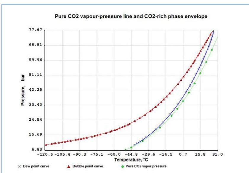
Figure 1: Pure Carbon Dioxide vapour pressure line and  $\text{CO}_2$ - $\text{CH}_4$  mixture
