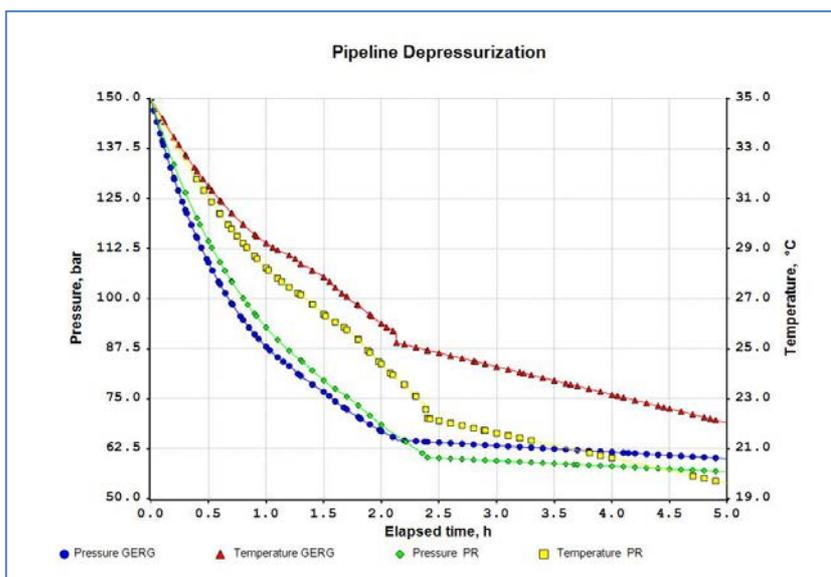
Figure 5: Pipeline depressurization – Pressure and temperature profiles for PR and GERG models
