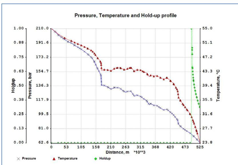
Figure 4: Pressure and temperature change – Two phases transport case
