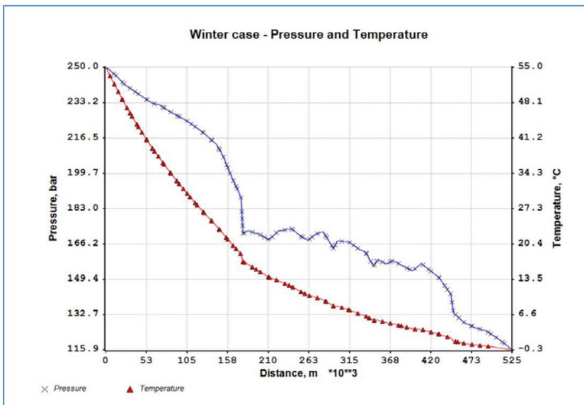
Figure 3: Pressure and temperature profile – Single phase transport case
